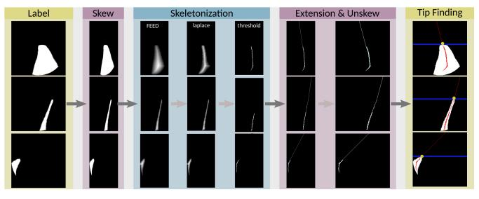
**Fig. 6.** Tool tip identification procedure. Pink blocks demonstrate the skew/unskew steps to amplify vertical height of the label. The blue block shows the intermediate results of the skeletonization step. The right most column denotes the mathematical derivation of the tool tip (yellow), the intersection of the skeleton (red), and the nearest nonintersecting horizontal line (blue).
