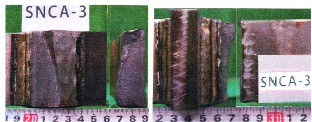
Fig.12 Fracture surface and pass after fatigue test (SUS329J3L-clad : Non load-carrying, As-welded) (SNCA-3 : 120N/mm 2 , 4.37×10 5 cycles)
