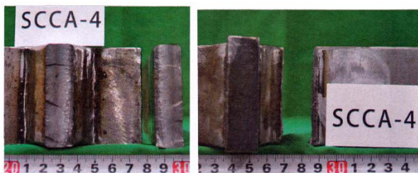
Fig.4 Fracture surface and pass after fatigue test (SUS329J3L-clad : Load-carrying, As-welded) (SCCA-4 : 170N/mm 2 , 5.53×10 5 cycles)
