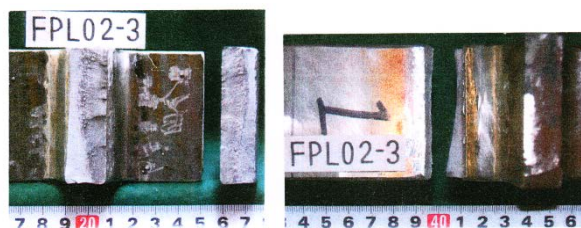
Fig.6 Fracture surface and pass after fatigue test (SUS316L-clad : Load-carrying, As-welded) (FPLO2-3 : 398N/mm 2 , 1.38×10 5 cycles)
