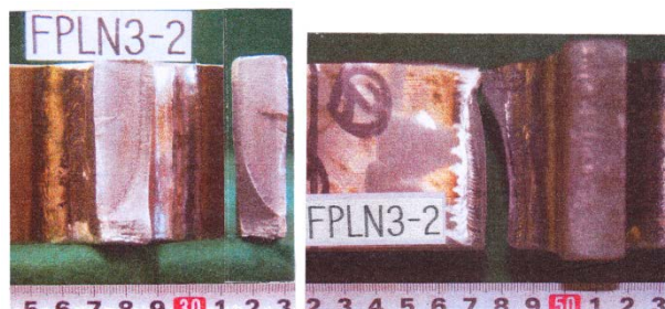
Fig.16 Fracture surface and pass after fatigue test (SUS316L-clad : Non load-carrying, TIG arc) (FPLN3-2 : 200N/mm 2 , 1.09×10 6 cycles)
