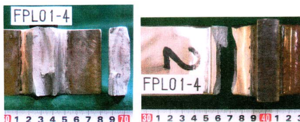
Fig.7 Fracture surface and pass after fatigue test (SUS316L-clad : Load-carrying, Grinding) (FPLO1-4 : 350N/mm 2 , 4.54×10 5 cycles)
