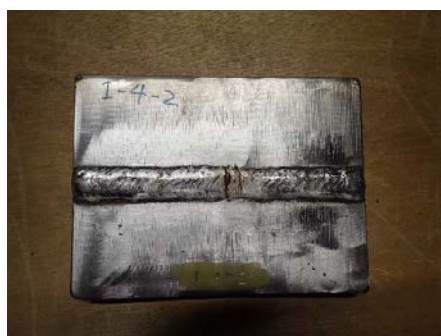
a) View of Transverse Crack
