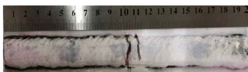
b) Result of Penetrant Test
