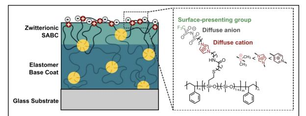
Figure 1. Marine fouling-resistant coatings are prepared using the surface-active block copolymer (SABC) approach where a thin layer of functional polymer is tethered to a thick elastomer base. This surface layer is functionalized with diffusely-charged zwitterionic groups and a fluorinated pendant end to drive surface segregation of the zwitterions. This work studies the effect of cation size by replacing the red cationic group with either ammonium, imidazolium or pyridinium.
