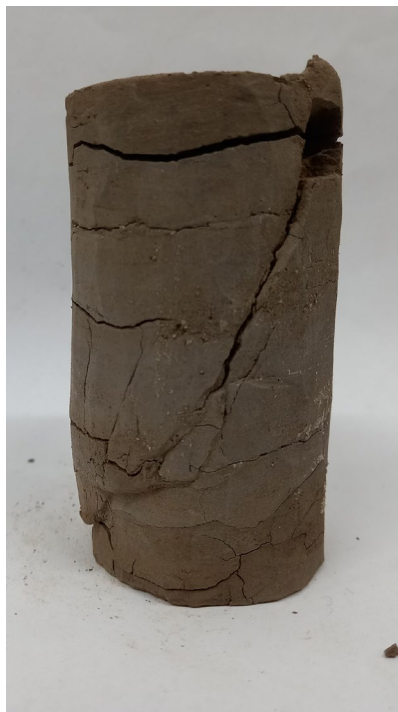
Advanced experimental testing on unsaturated soil subjected to drying-wetting cycles.
