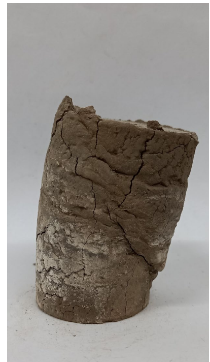
Advanced experimental testing on unsaturated soil subjected to drying-wetting cycles.
