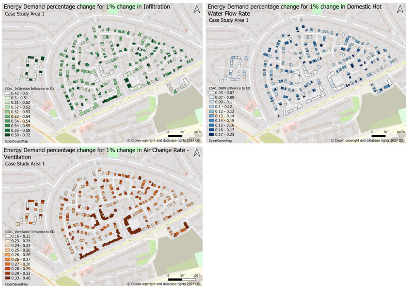
Figure 4 Impact on Annual Residential Building Energy Demand for 1% change in the under-test Program Type building parameters in CSA1.
