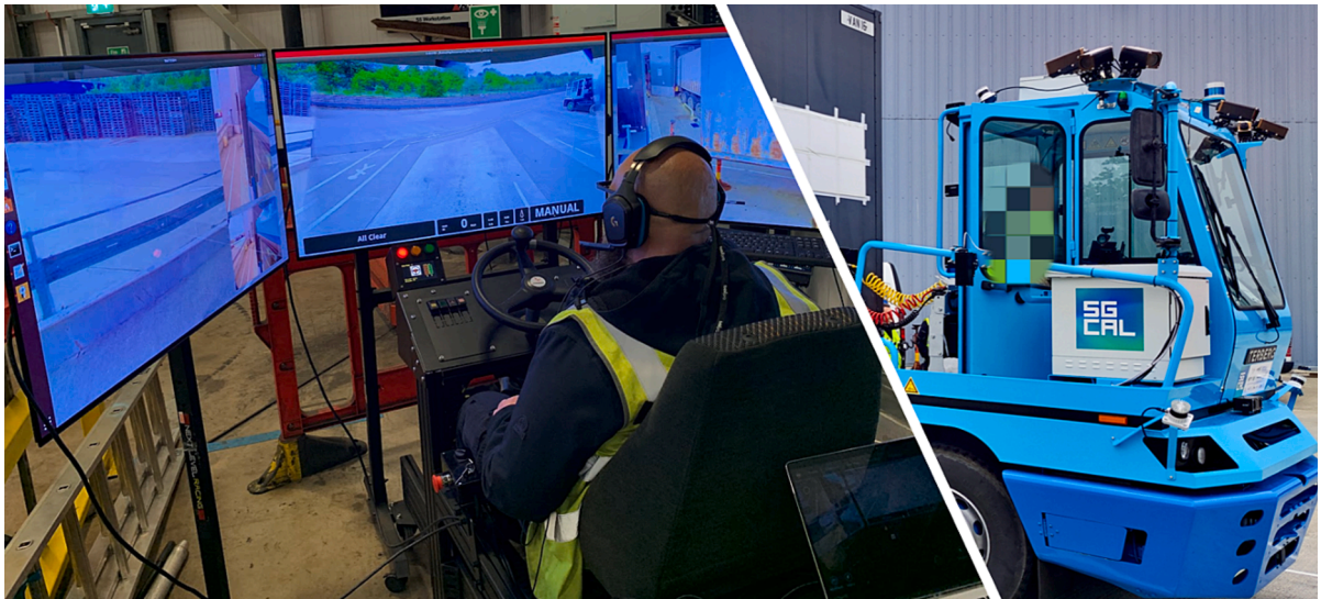
Fig. 2. An example of a remote driver operating a teleoperation workstation for remote driving (left) of a 5G-enabled Level 4 automated vehicle (right) in the DCMS 5G Connected Automated Logistics project.
