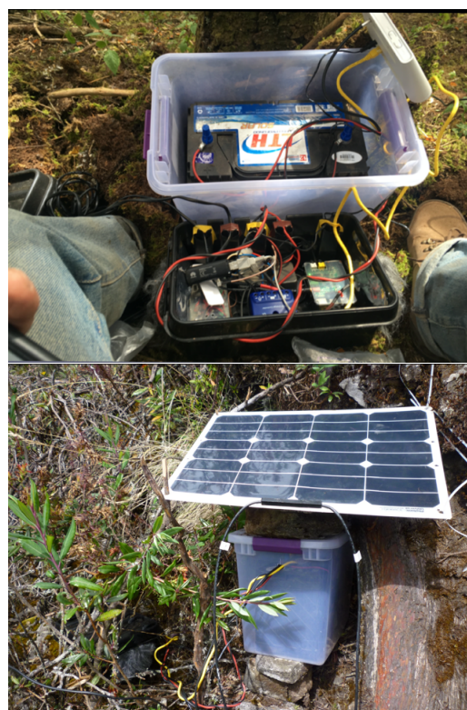
Figure 2. Above: Streambox and battery with wireless router in the Cerro Pelón UNESCO Biosphere Reserve in the State of Mexico. Below: Streambox, battery housing and solar panel in initial installation position in the Cerro Pelón UENESCO Biosphere Reserve.
