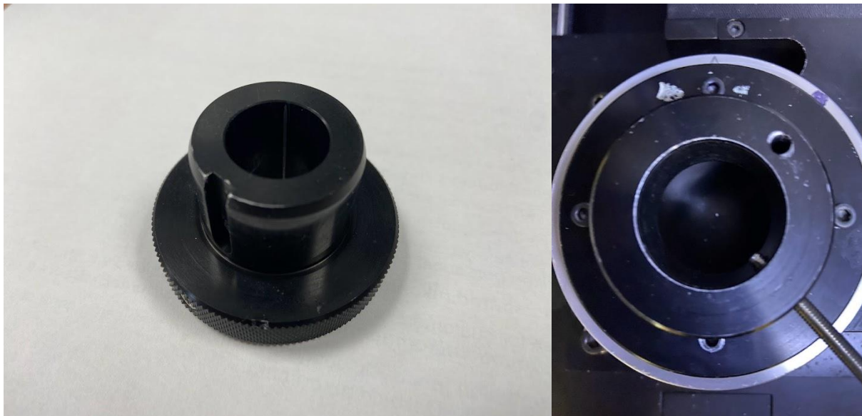
Figure 3-4 shows the underside of the standard Nikon stage, note the keyway on the left of the cylinder.
