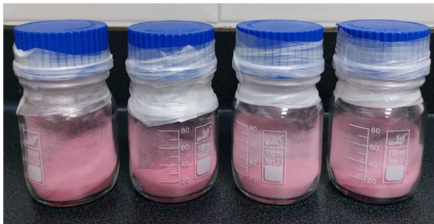
Fig. 2 Images of foamed cornelian cherry powder samples dried by convective drying at 50, 60, 70, and 80°C (from left to right)
