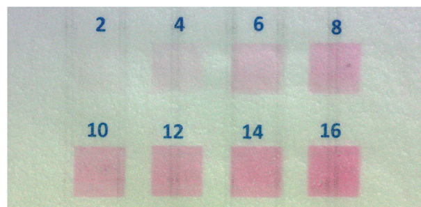
Figure 4. Inkjet-printed ODFs (2 cm 2 in size) containing escalating doses of propranolol hydrochloride printed onto edible rice paper. Reproduced with permission. [32] Copyright 2016, Elsevier.
