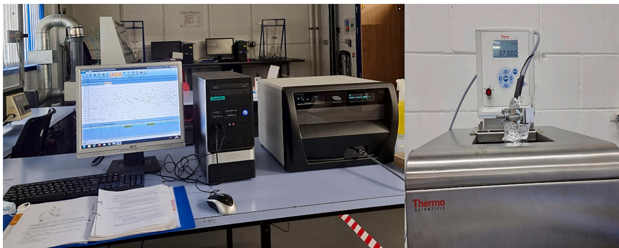
Fig. 7. Thermal conductivity setup attached to the thermal bath.
