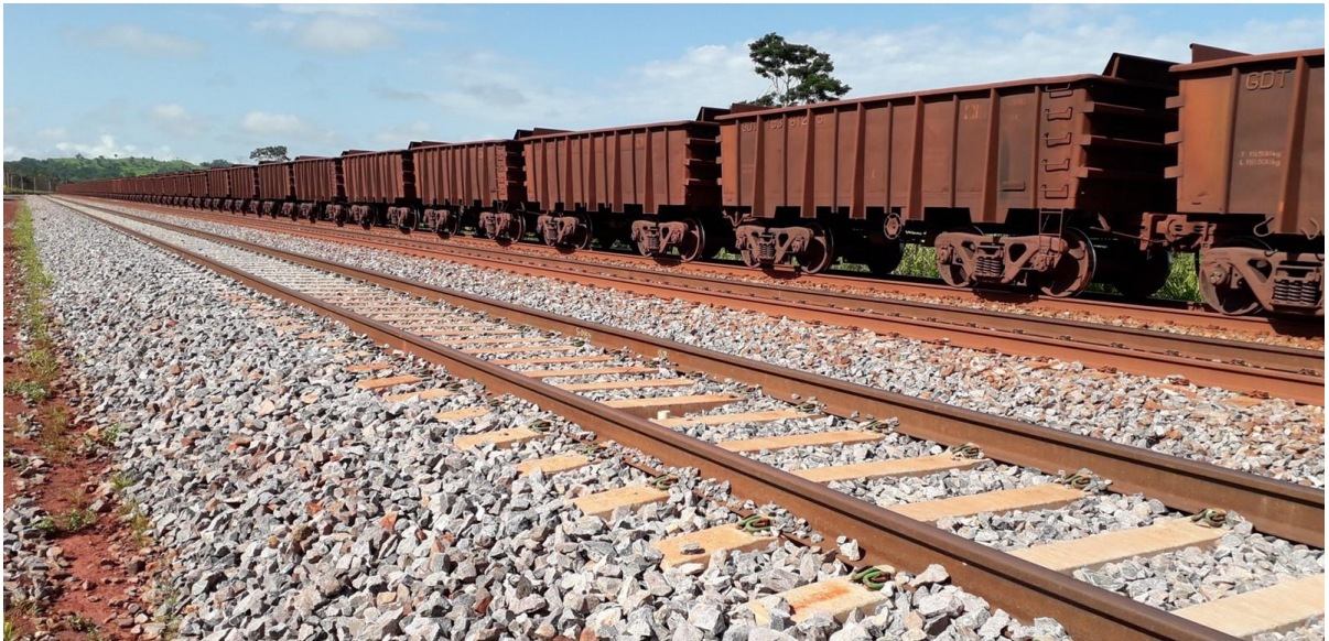
Figure 2.0-11. Typical iron ore train composition of a heavy-haul railway with unloaded wagons (8 distributed locomotives and 333 wagons).
