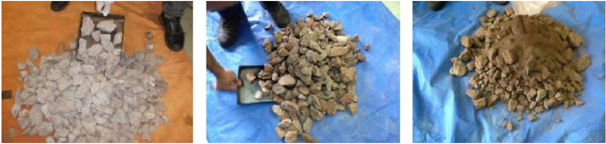
Figure 2.0-5. Examples of different ballast conditions: fresh ballast (right), recycled ballast (medium), and fouled ballast (left) (Costa 2016, and Costa et al. 2017).
