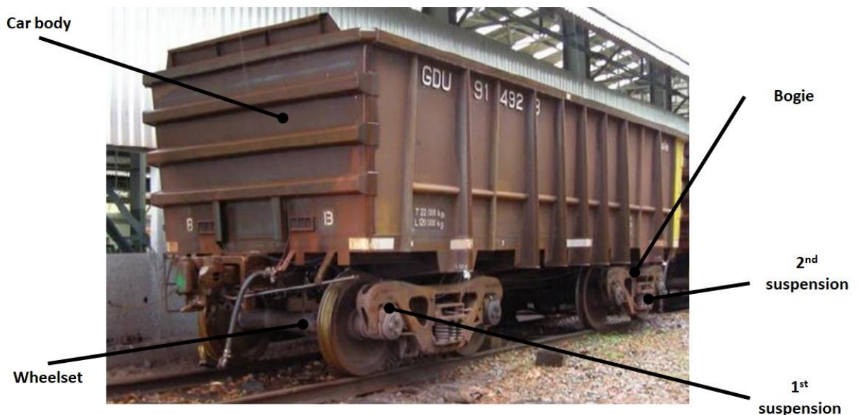
Figure 2.0-10. Key railway vehicle components and their respective position on a heavy-haul wagon framework (modified from Santos 2015).
