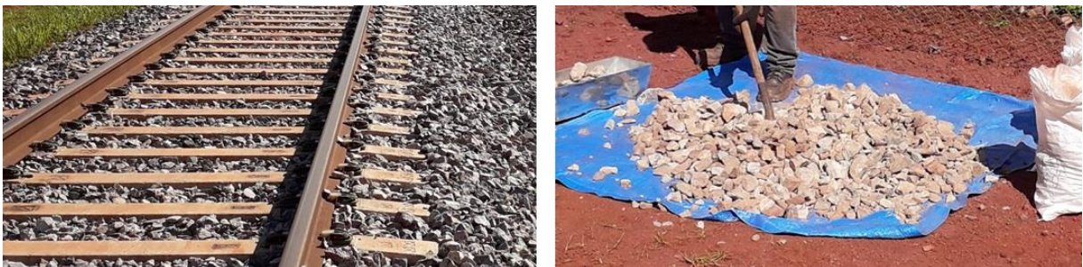
Figure 2.0-7. Typical ballast material of heavy-haul ballasted railway track: track view (left) and sample being quartered to be analyzed in laboratory (right).
