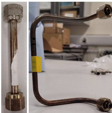
Figure 3.3: Initial (left) and final (right) reactor sections, with 80 and 354 mm, respectively.
