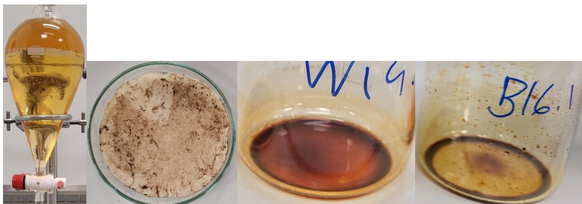
Figure 8.4: From left to right, examples of phase separation during solvent extraction, and evaporated samples of solids, WSO, and DSO.
