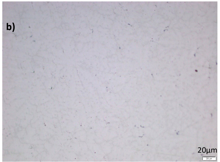
Figure 66. a) and b) show the cross-section and microstructure of AZ91_T650_S120, respectively.
