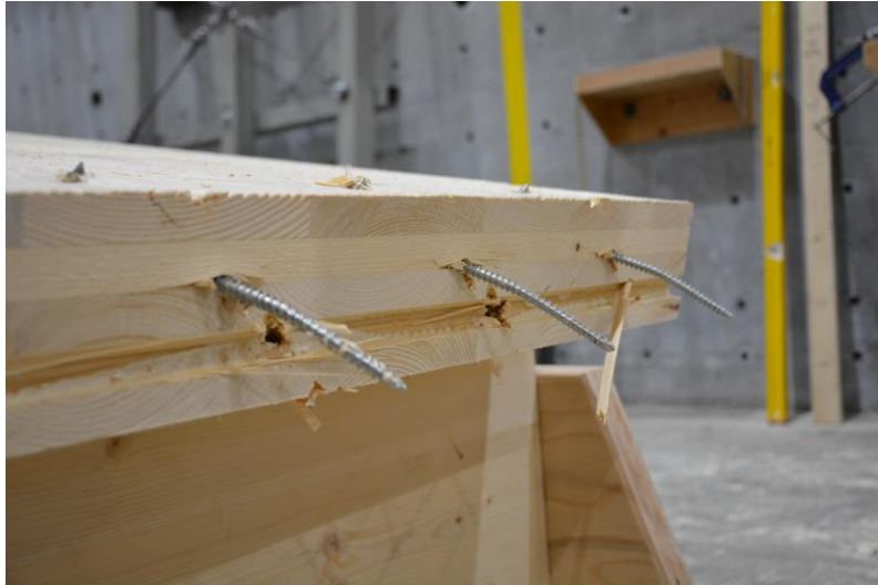
Figure 6. 24 Double incline butt joint screw withdrawal failure
