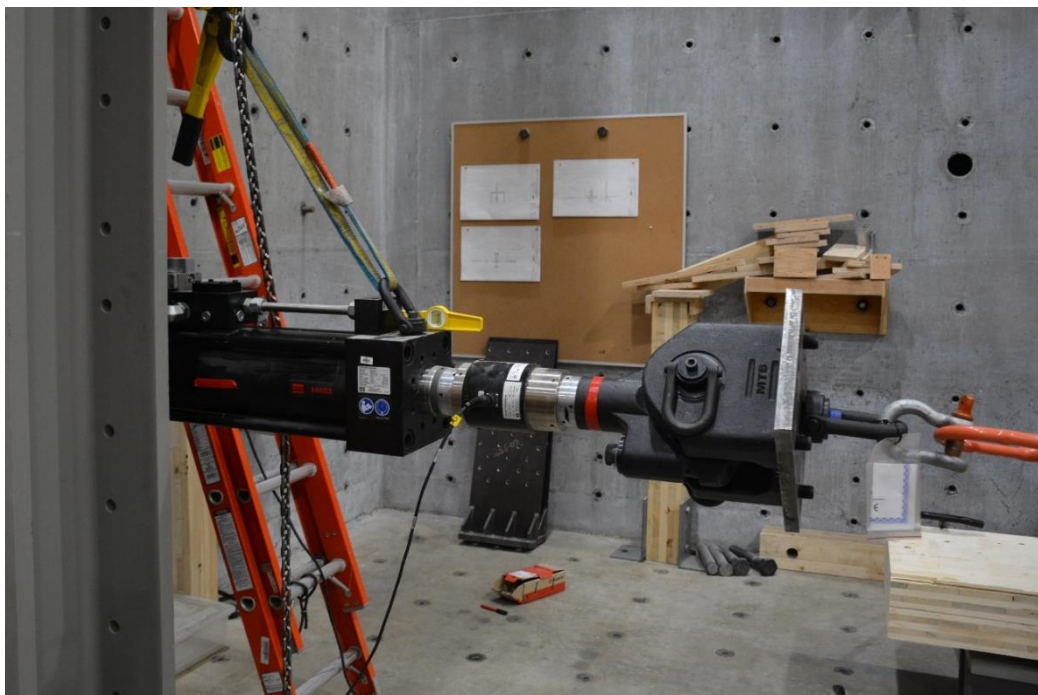
Figure 5. 6 Experimental Setup B horizontal actuator installation
