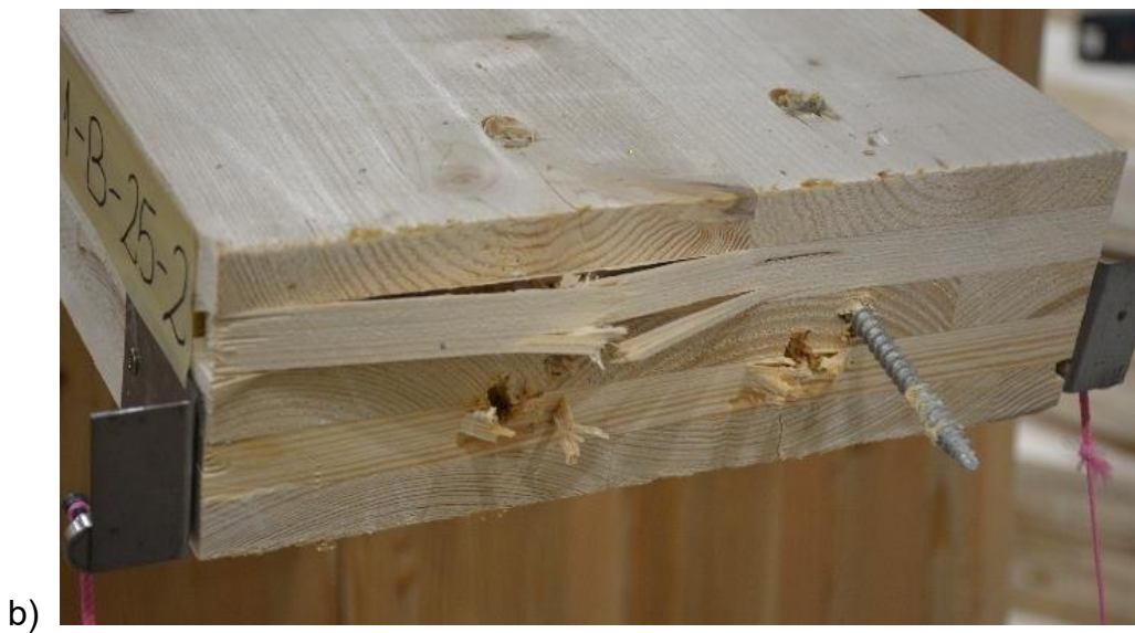
Figure 5. 14 Butt joint component tested to maximum stroke (a) and to failure (b)
