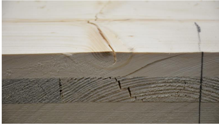
Figure 6. 22 Rolling shear failure with tensile failure at the top over the knots
