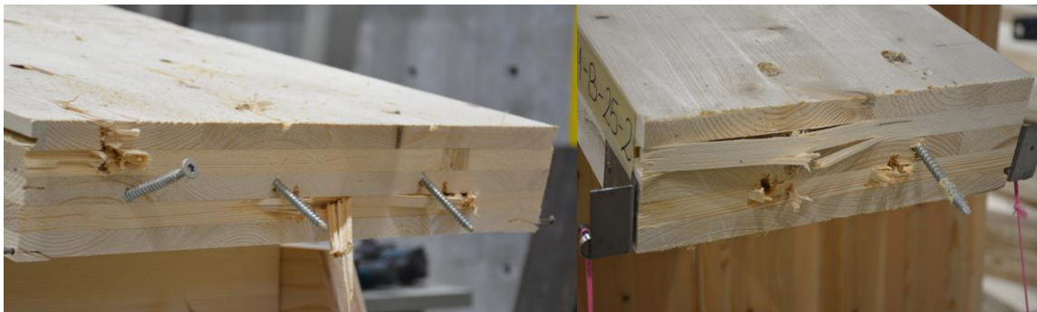
Figure 7. 5 Side by side comparison of the full span (left) and component (right) tests
