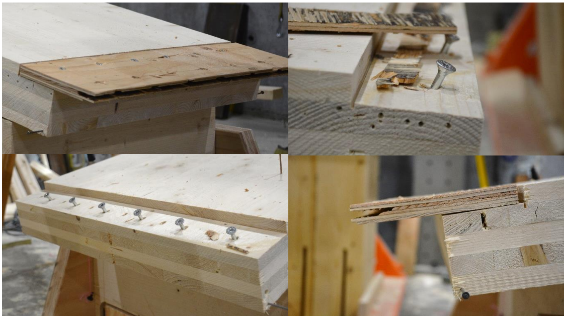
Figure 6. 26 Examples of the spline failure
