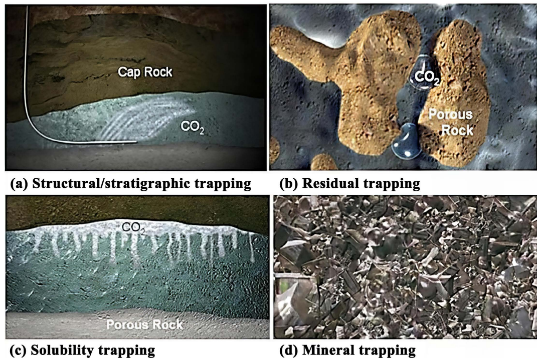
Figure 3. Illustrate the major 4 CO 2 trapping subsurface systems (Zhao et al., 2014).
