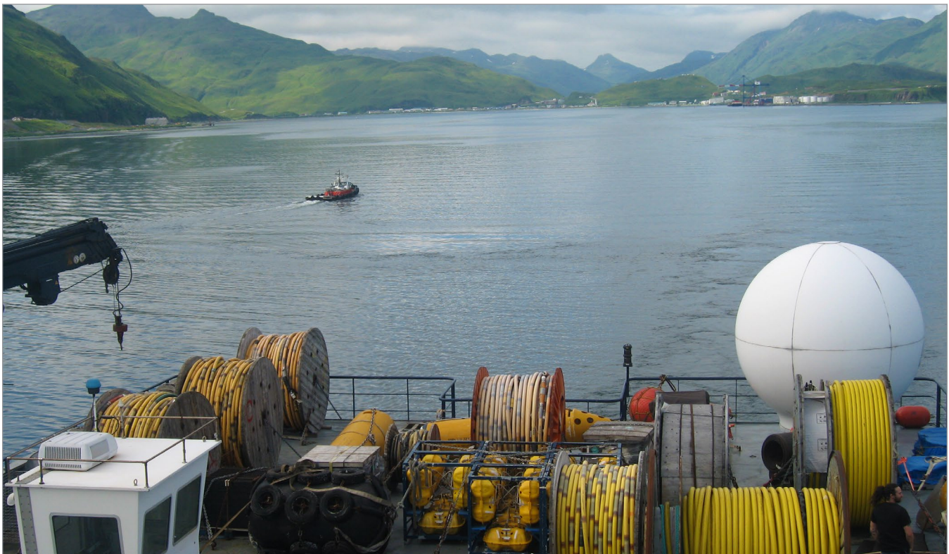
The rear deck of R/V Marcus G. Langseth as it departs Dutch Harbor, Alaska to collect data in the Bering Sea. The vessel collected the multichannel seismic data necessary to apply the sediment thickness formula in the Bering Sea Region. Image courtesy of Jennifer Jencks.
