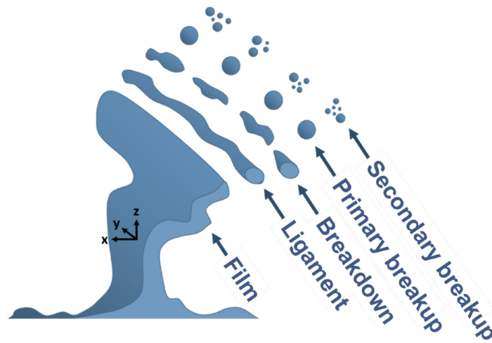
Figure 2.2. Droplet formation from wave instability of thin liquid films.
