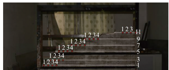
图7 边坡测点布置
