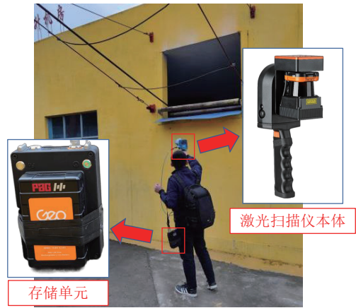
图 2 扫描现场与三维激光雷达 Fig.2 Field scanning and 3D lidar
