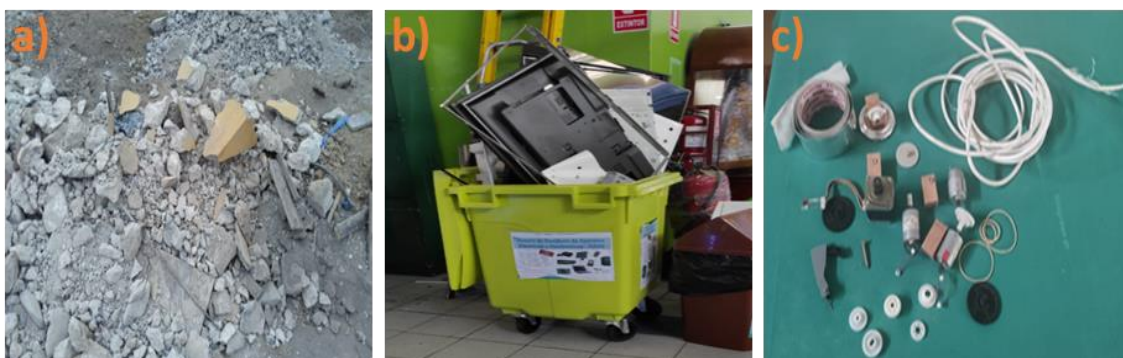
Figure 1: Wastes collected: a) Construction and demolition wastes; b) Waste electrical and electronic equipment; c) Waste electrical and electronic equipment used
