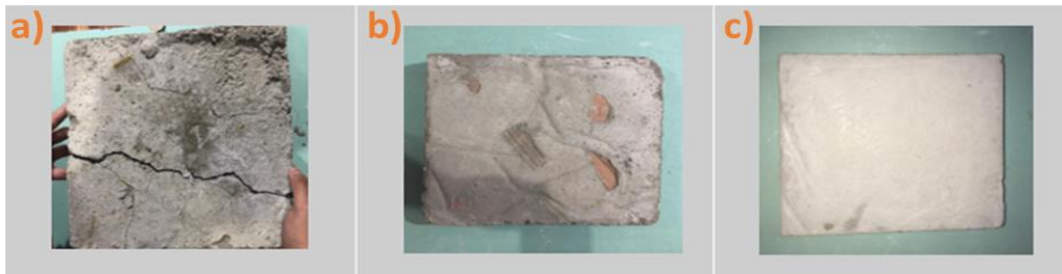
Figure 4: Composition of slabs: a) 70% CDW + 30% virgin material; b) 50% CDW + 50% virgin material; c) 25% CDW + 75% virgin material
