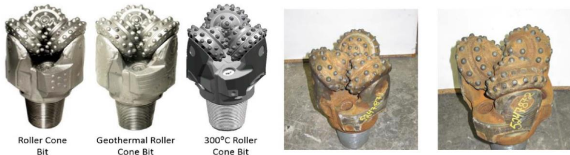
Figure 2 – Different Roller Cone Bit (right). Effect of temperature (300 °C) and bit wearing in IDDP-2 well (left) (Stefanson, et al., 2018)
