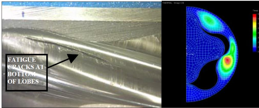
Figure 4 – Fatigue cracks and thermal hysteresis build up in PDM motors (Delpassand, 2017)
