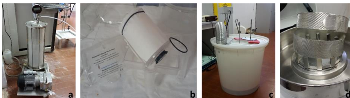
Figure 1: a) Vacuum pump with washing water tank, b) drum filter with filter material, c) water bath system for digestion, d) ultracentrifuge mill sieve with 0.15 mm and 0.08 mm meshes.
