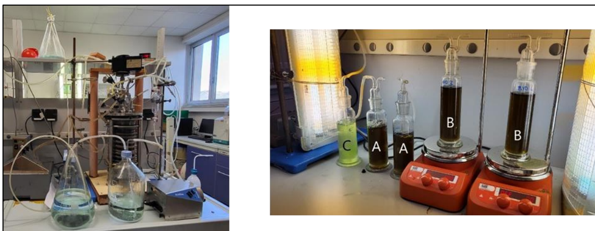
Figure 1: 6-L bioreactor used for OFMSW anaerobic digestion (left hand side). C. vulgaris cultures in 0.25-L bubble columns (C = control run, A = growth with digestate and continuous air supply, B = growth with digestate and biogas) (right hand side).
