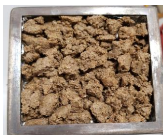
Figure 1: Gasification test rig (Cone calorimeter) Figure 2: Draff sample for gasification (sample weight 82 g)
