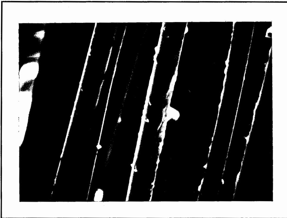
Figure 100. Fiber Surface, 1 Hz, 1093°C, 137.9 MPa, 625X
