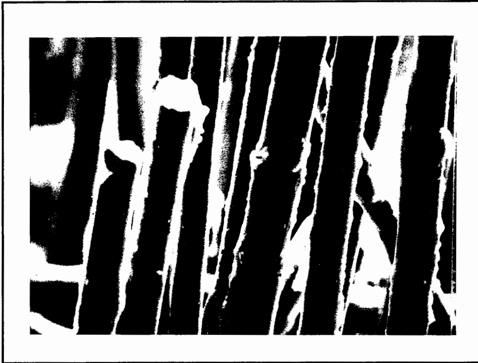
Figure 101. Fiber Surface, 1 Hz, 1093°C, 96.53 MPa, 575X
