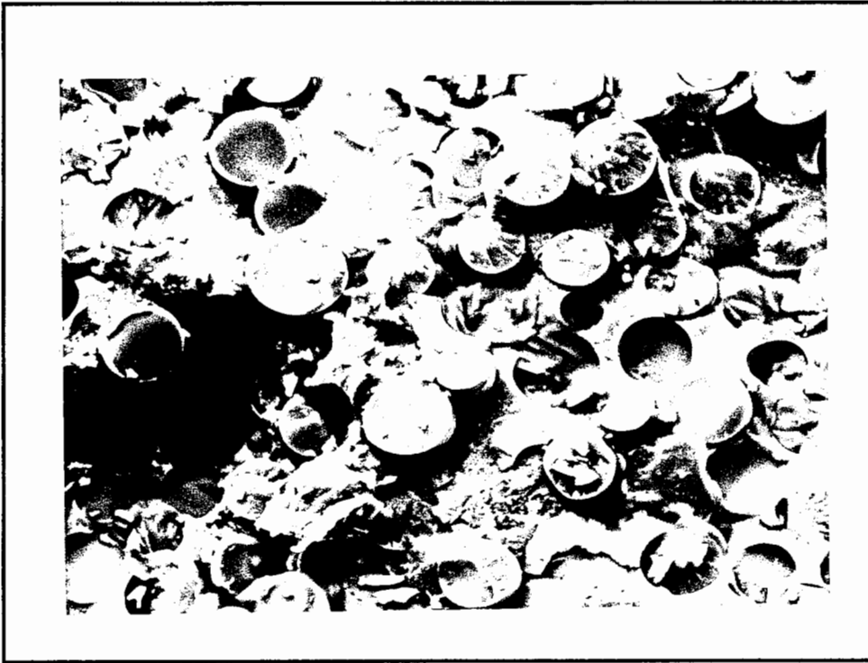
Figure 95. Fracture Surface, 10 Hz, 1093°C, 720X
