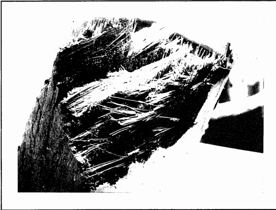
Figure 74. Fracture Surface, Monotonic Tensile, 566°C, 15.2X
