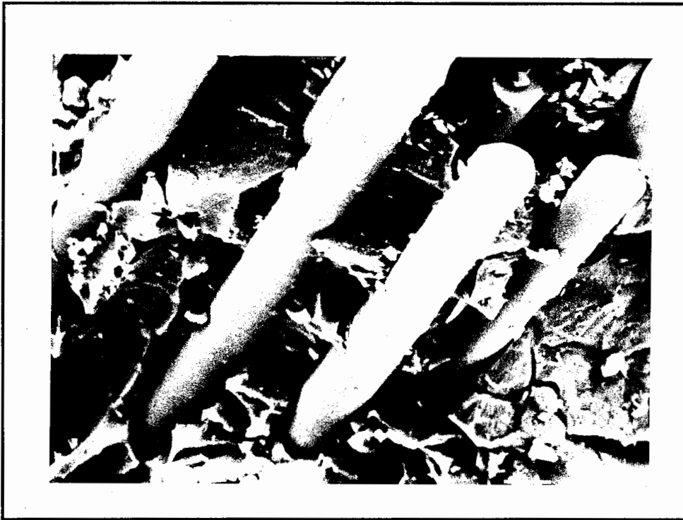
Figure 79. Fiber Surface, 10 Hz, 566°C, 137.9 MPa, 685X
