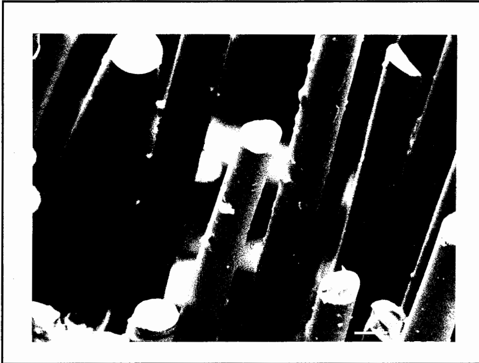
Figure 94. Fiber Surface, 10 Hz, 1093°C, 96.53 MPa, 855X
