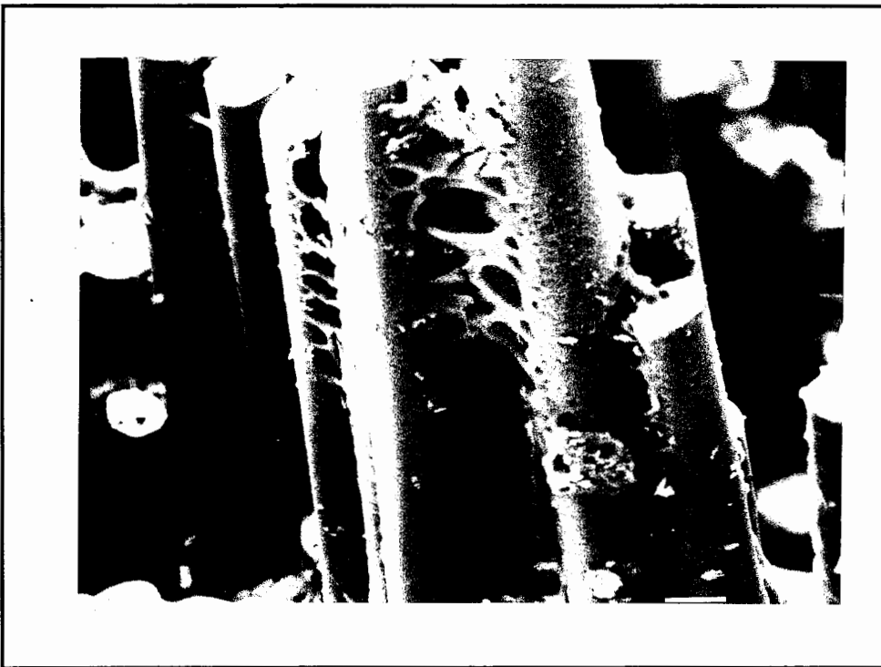
Figure 80. Fiber Surface, 10 Hz, 566°C, 103.43 MPa, 470X
