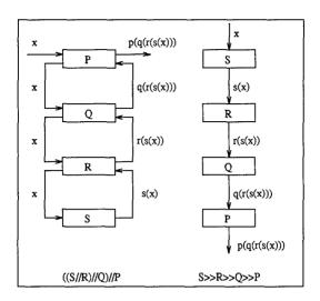
Figure 6.14 Comparison of Layered versus Pipelined Operation
