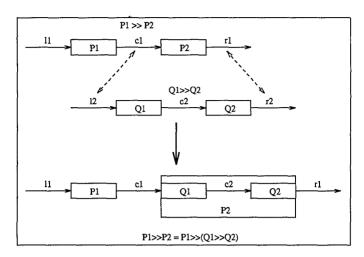
Figure 6.10 Recursive Application of Pipeline Structuring Specification
