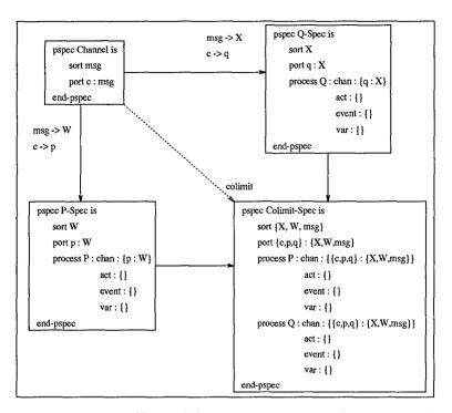
Figure 6.5 Using Channel Specifications to Unify Port Symbols
