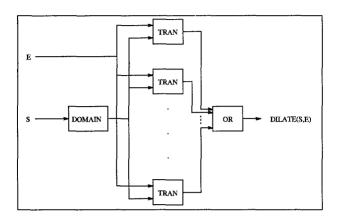
Figure 8.8 Block diagram of DILATE (33:342)
