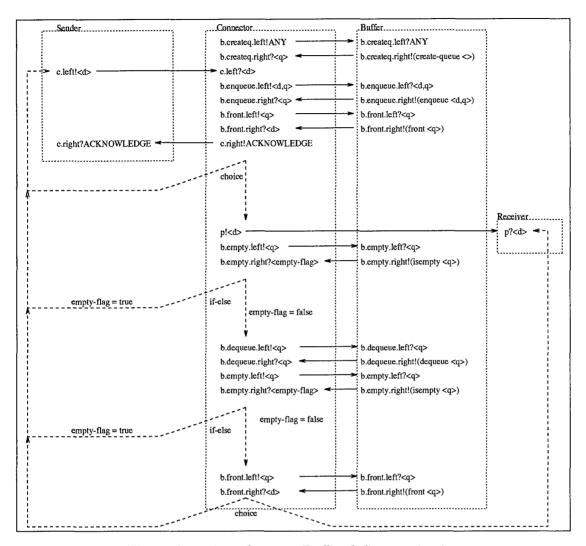
Figure C.3 Asynchronous Buffered Communication
