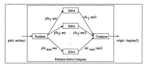
Figure 8.12 Block diagram of Partition-Solve-Compose
