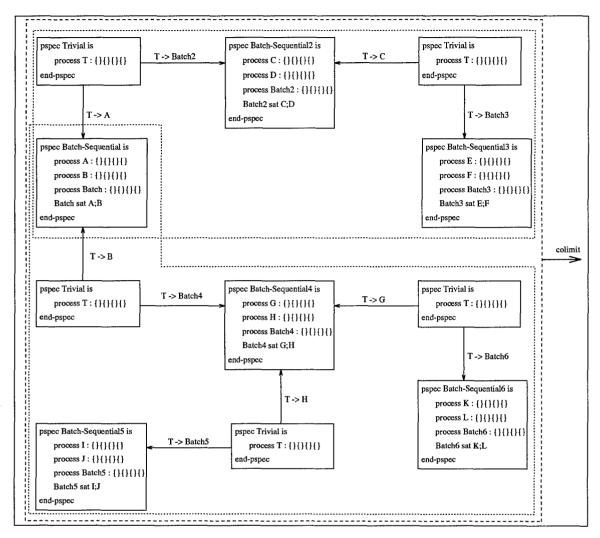
Figure 6.17 Creation of a Seven Segment Batch-Sequential Design
