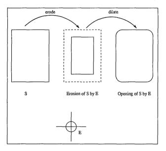
Figure 8.10 Opening in terms of dilation and erosion (33:334)
