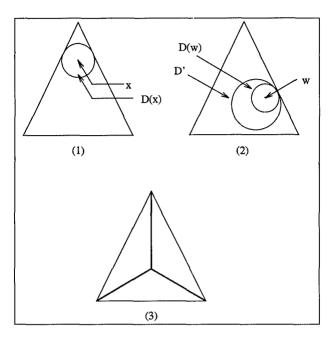
Figure 8.3 Determining skeleton for isosceles triangle (33:352)
