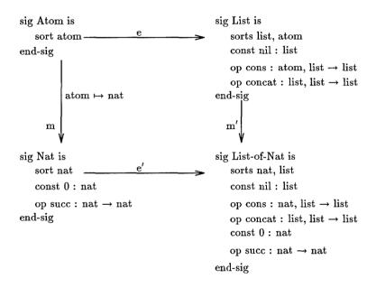
Figure 3.4 Instantiation of a Signature for a List of Natural Numbers
