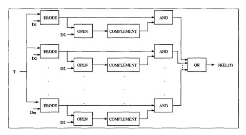
Figure 8.6 Block diagram of SKEL (33:355)
