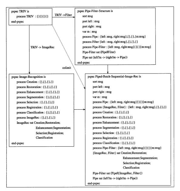
Figure 8.1 Piped-Batch Sequential Image Recognition
