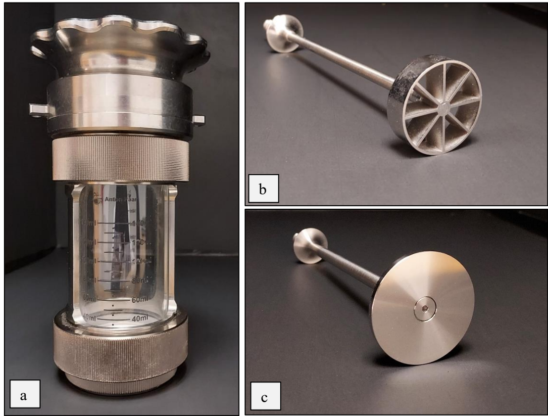
Figure 4.1: Components of the flow cell for the Warren Springs and Wall friction tests. (a) – glass flow cell container. (b) – Warren Springs geometry piece. (c) – Wall friction compression piece.
