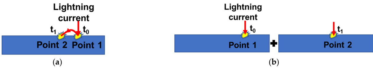
Figure 10. Schematic of swept stroke FE models: (a) the swept stroke model and (b) the superposition model.
