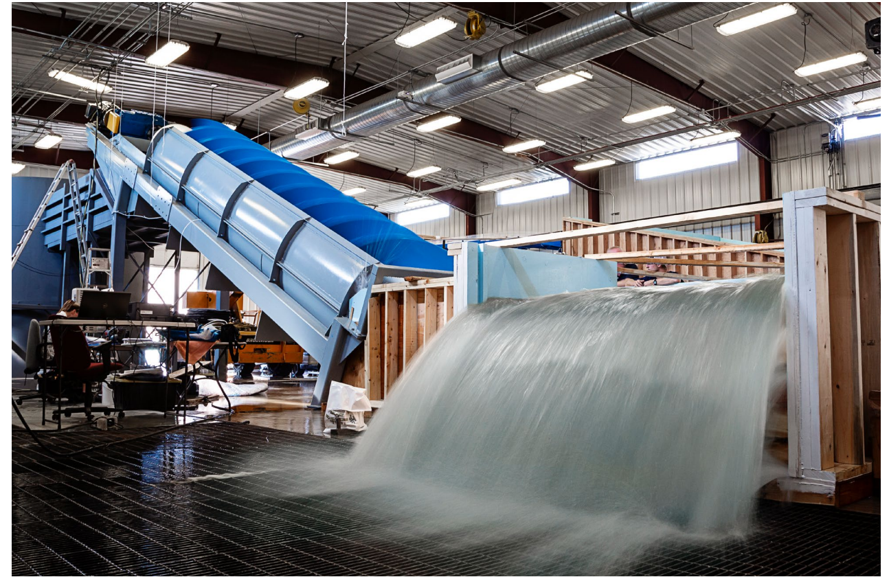
Utah Water Research Lab engineers are testing a hydrodynamic turbine modeled after Archimedes’ screw.
