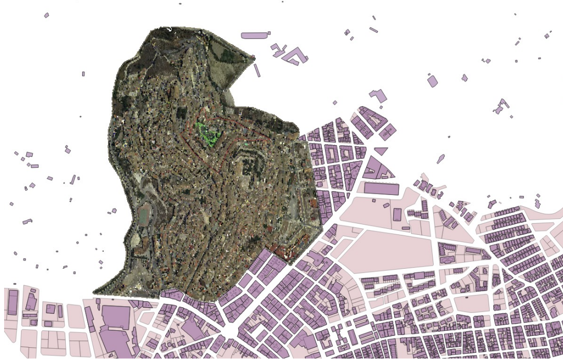
Fig. 5. Lidar point cloud of the historical centre and cadastral data overlapped and geo-referenced in QGIS.
