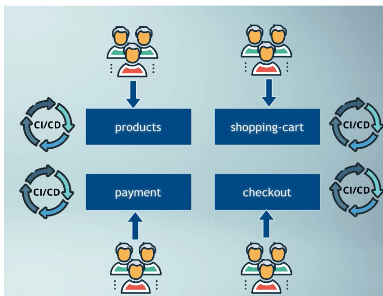
Figure 2.5: Example of an e-commerce software application using microservice architecture (retrived from [Janashia 2022])
