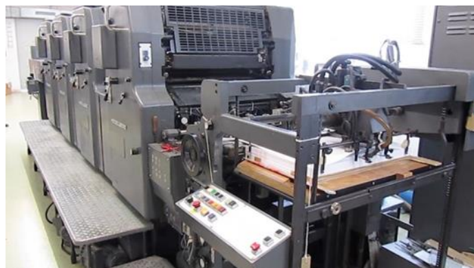
Figure 11 - Typical lithography machine with multiple color sequences
