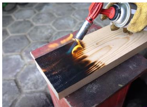
Figure 2. Burn Process with a Blowtorch [Source : Youtube Video [6]]
