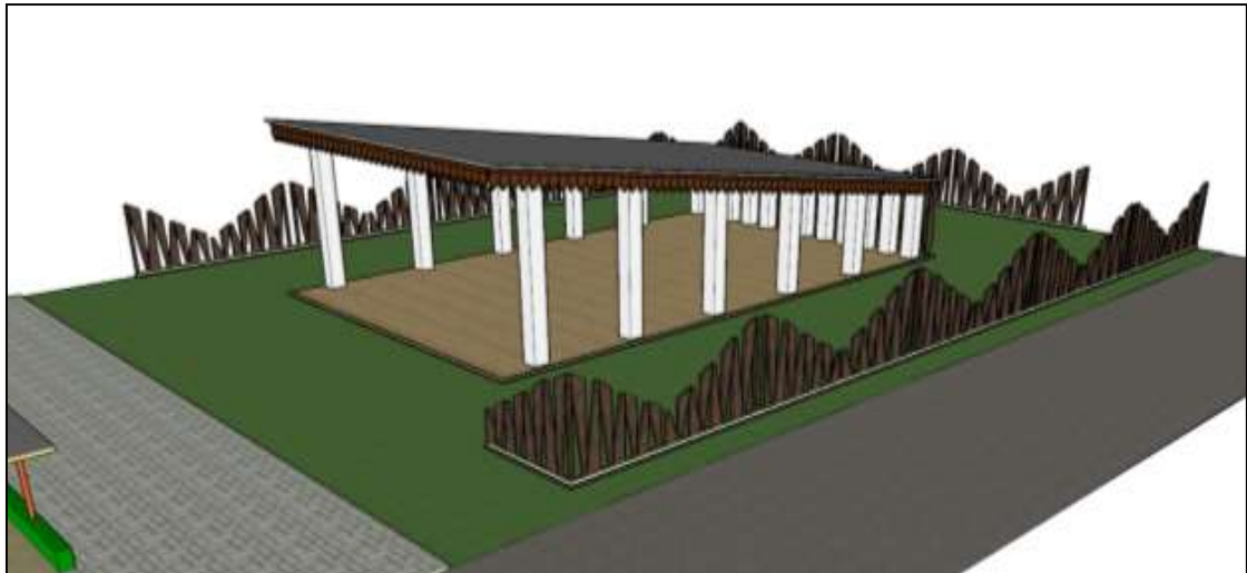
Figure 3. Tagog anjing roof model to articulated Sunda traditional architecture (picture source: Widia Nur Intan Paramita, joint research Pancasila University)
