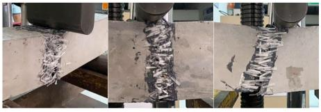
Fig. 6 - Failure after repaired (1st Method)
