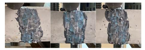
Fig. 8 - Failure after repaired (3rd Method)
