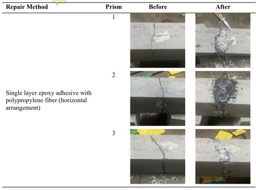
Table 2 - Image of before and after concrete prism repaired
