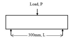
Fig. 2 - Schematic drawing of three-point bending test
