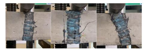
Fig. 7 - Failure after repaired (2nd Method)
