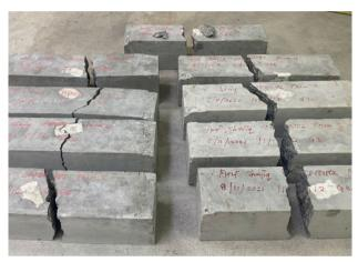
Fig. 5 - Concrete failure before repaired
