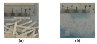
Fig. 1 - Fiber materials (a) polypropylene fiber; (b) surgical mask fiber
