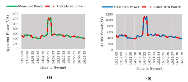
Fig. 7 Measured power and calculated power of (a) Apparent power; (b) Active power of the residential building
