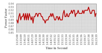
Fig. 8 Measured power factor of the tested residential building
