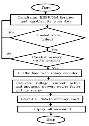
Fig. 5 Flow chart of a smart metering system
