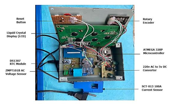
Fig. 3 Development of smart energy meter
