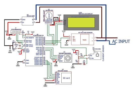
Fig. 2 Circuit diagram of the smart energy meter
