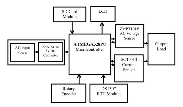
Fig. 1 Block diagram of a smart metering system
