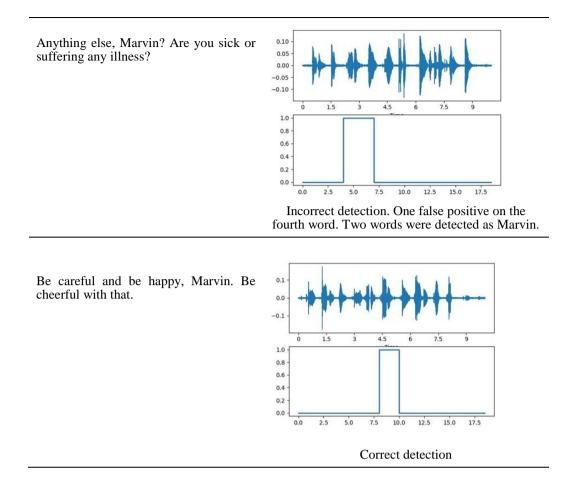
For noisy background (Session 2), the detection is accurate for up to 50 dB for practical usage. This means that ambient noise of more than 50 dB would severely affect the detection of the wake word due to the presence of unwanted signals in both amplitudes and frequencies. The detection would improve by speaking very loud or close to the microphone. Detection results for up to 50 dB noise are shown in Figure 3 to 6. Only selected results are shown.
