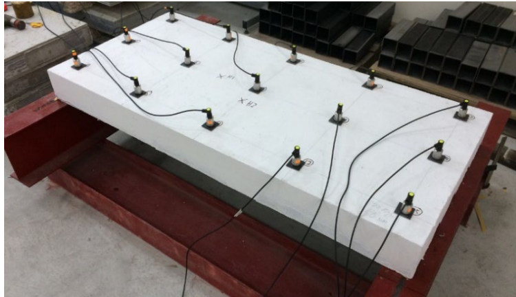
Fig. 2 - Location points for accelerometer and external loading
