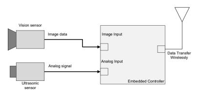
Fig. 2 - Block diagram of smart sensory system
