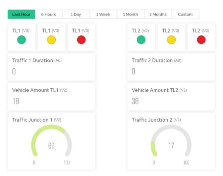
Fig. 7 - The developed real-time IoT dashboard
