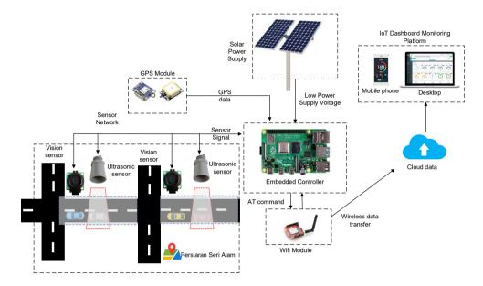
Fig. 1 - Smart network adaptive traffic light system via Internet of Things (IoT)
