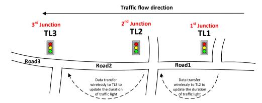
Fig. 4 - Traffic light duration adjusts prioritized according to traffic flow and location wirelessly
