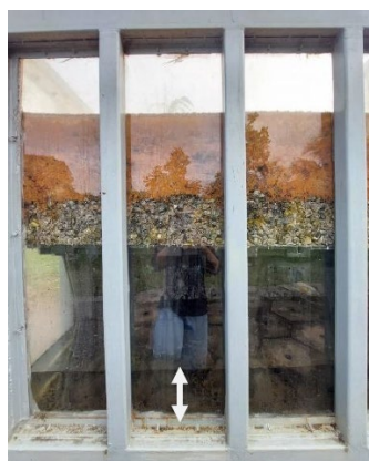
Fig. 6 - By measuring the water level (shown with white arrow), the volume of water detained
