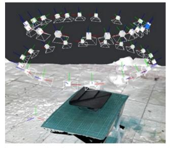
Fig. 2 - Final 3D reconstruction of part Y and its position and orientation of camera
