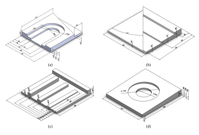
Fig. 1 - Isometric view for test piece (a) X; (b) Y; (c) G, and; (d) H
