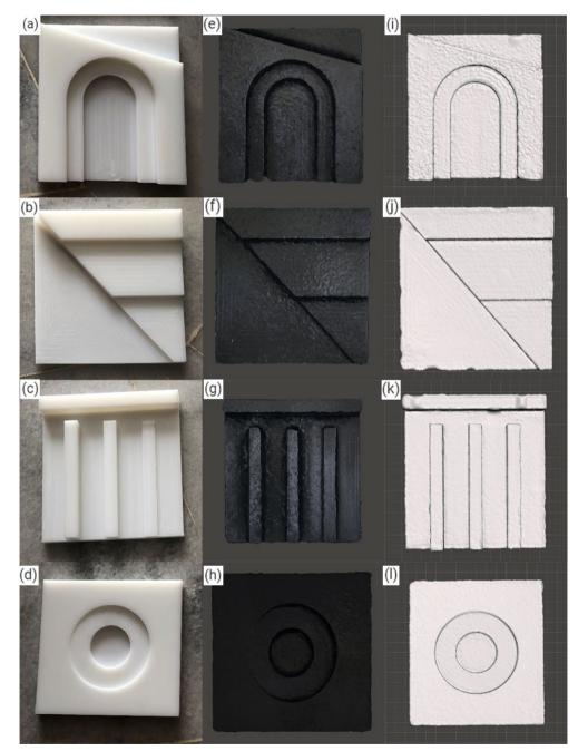
Fig. 3 - Comparison among fabricated test pieces, reconstructed 3D models by low and high-cost 3D scanning system (a)~(d) original test pieces X, Y, G and H, respectively; (e)~(h) reconstructed 3D models using photogrammetry technique by Meshroom software, and; (i)~(l) reconstructed 3D models using high-end 3D scanner by VXelements software
