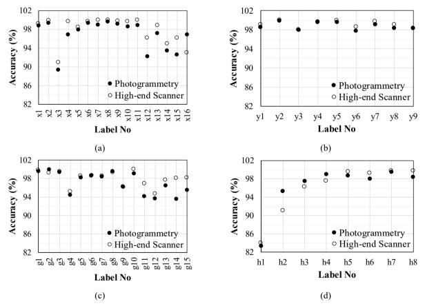
Fig. 4 - Comparison of dimension accuracy between mobile photogrammetry and high-end scanner for test piece (a) X; (b) Y;(c) G, and; (d) H
