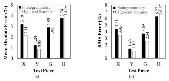
Fig. 5 - Comparison of (a) mean absolute error (MAE) and; (b) root-mean-square error (RMSE) between mobile photogrammetry and high-end scanner
