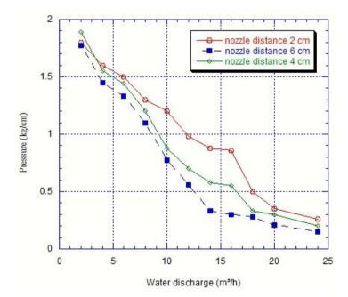
Fig. 6 - The graph of relationship between water discharge and pressure at various nozzle positions
