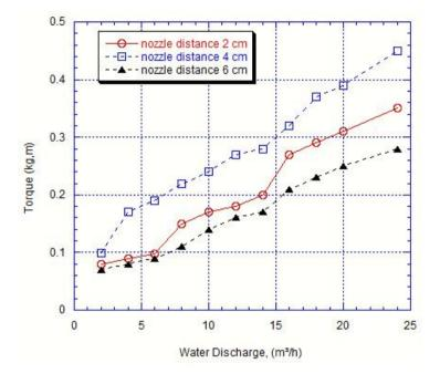
Fig. 5 - The graph of relationship between water discharge and torque at various nozzle positions
