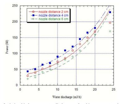
Fig. 7 - The graph of relationship between water discharge and turbine power at various nozzle positions
