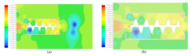
Fig. 8 - Fluid flow at a nozzle distance of 2 cm (a) pressure 0.26 kg/cm<sup>2</sup>; (b) pressure 1.8 kg/cm<sup>2</sup>
