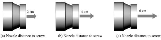
Fig. 2 - Test design position nozzle distance to screw turbine (a) 2 cm; (b) 4 cm; (c) 6 cm
