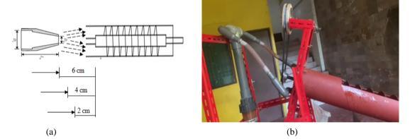
Fig. 3 - Experimental conditions (a) complete condition nozzle to screw distance; (b) side view of nozzle position on pico-hydro test equipment
