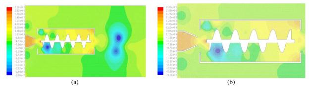
Fig. 9 - Fluid flow at a nozzle distance of 4 cm (a) pressure 0.2 kg/cm<sup>2</sup>; (b) pressure 1.89 kg/cm<sup>2</sup>
