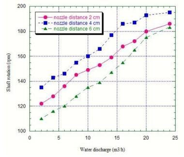
Fig. 4 - Graph of discharge relationship with shaft rotation
