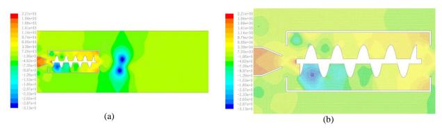
Fig. 10 - Fluid flow at a nozzle distance of 6 cm (a) pressure 0.15 kg/cm<sup>2</sup>; (b) pressure 1.77 kg/cm<sup>2</sup>
