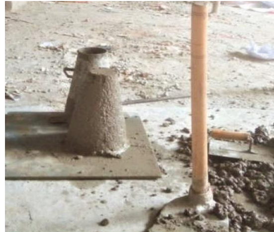
Fig. 3 - Slump test of concrete (True slump)
