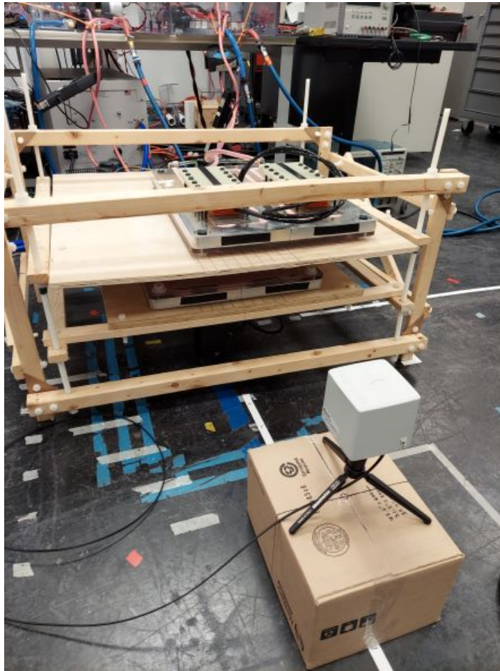
Figure 5.54: Field measurement setup of the Gen. 2 demonstrator. Here a box was used to elevate the probe to the middle of the airgap and tape was placed with markings at distances of 60 cm, 80 cm, and 100 cm on the X and Y axes.
