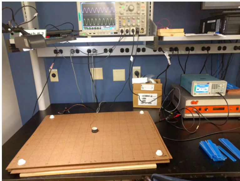
Figure 4.7: Surface field measurement of 6.6 kW coil: (a) Predicted surface B_z of coil. (b) Scaled measured surface B_z of coil. (c) Measurement setup with power amplifier.
