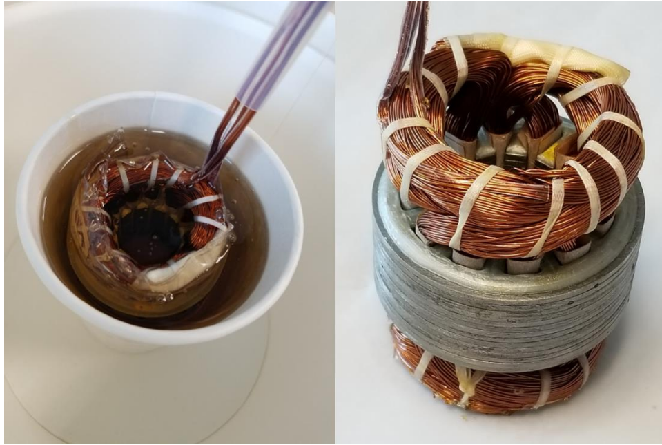
Figure 7.11: The stator assembly submerged in varnish (left); the stator assembly coated in varnish.
