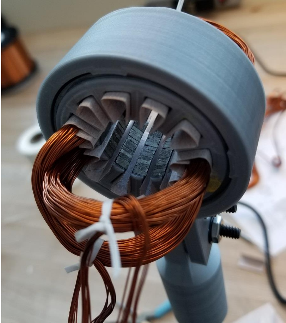
Figure 7.9: The motor undergoing the winding process.
