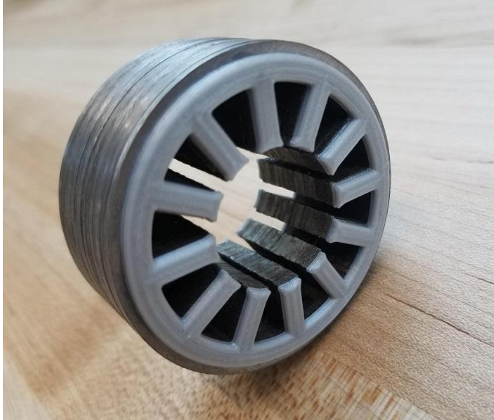
Figure 7.8: Stacked EDM sliced 3D printed Fe 3 Si laminates.
