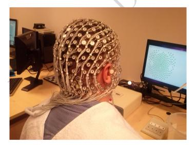
Figure 1. 256-electrode cap in EEG Laboratory
