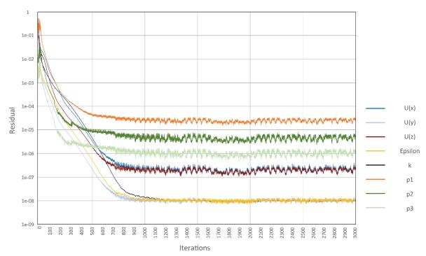
Figure 7. Residual Logarithmic graph for Morphology 2, Refine level 2.
