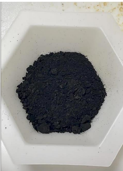
Figure 35. Manganese solid product with a purity of 46.99 wt.% generated during HNO 3 dissolution.
