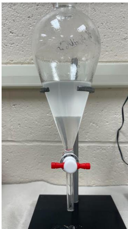
Figure 46. Stripping process developed for the extraction of cobalt from the loaded organic solution.
