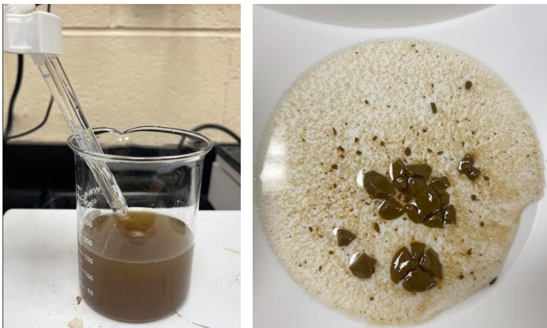
Figure 25. Solids precipitated during the pH adjustment of the SX feed solution.
